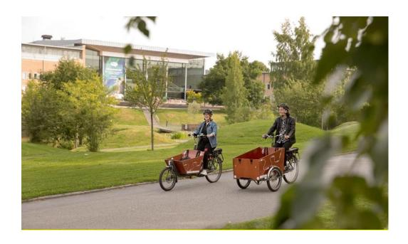
The super bikeway in Umeå municipality is a bicycle path with a higher standard than other conventional bicycle paths in Sweden. The superiority is in its dimensions, secured crossings, separation of bikes and pedestrians and in its interconnections to other bike paths. The bicycle path is also straighter and wider than the conventional bicycle path.
